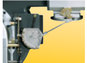
Example of the variable profile cam on RS 70-100-130 burners.
